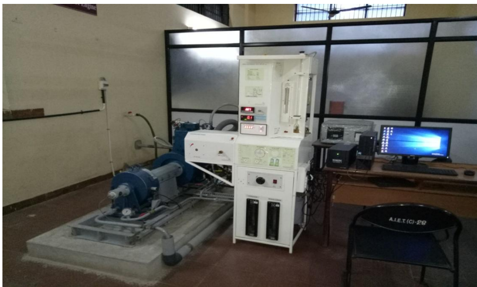
Fig.1 Pictorial view of CRDI VCR C.I.Engine test rig
